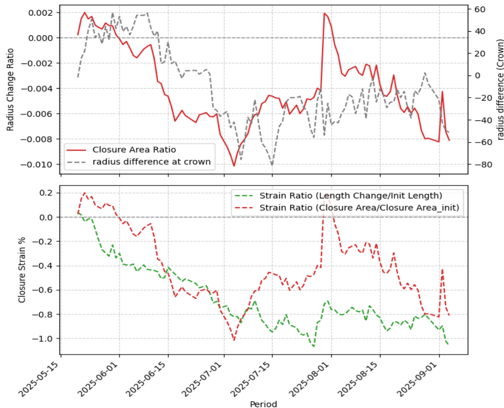
Figure 8 (Top) The closure strain calculated by using ratio of change of radius to original radius at crown compared to the average closure by using closed area of initial and final state. (Bottom) the closure strain calculated by using ratio of change of circumferential length to original length of segment curve.
