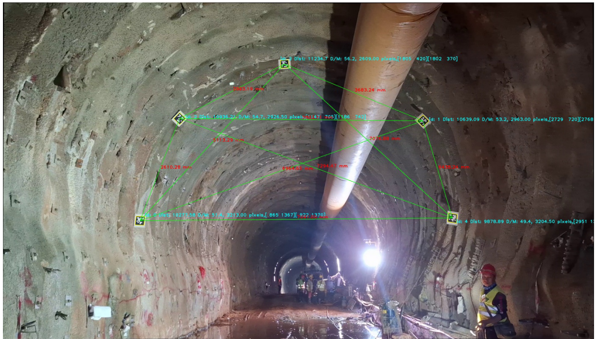
Figure 5 The markers were installed after tunnel experienced ground squeezing.
